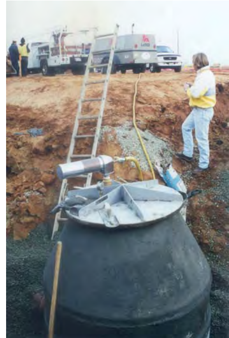
Example of our 1000-36 Vacuum Test Plate and our 1000-80 Venturi Vacuum Pump in use
