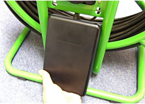
Slot Power Cell into frame and push upwards to lock in place
