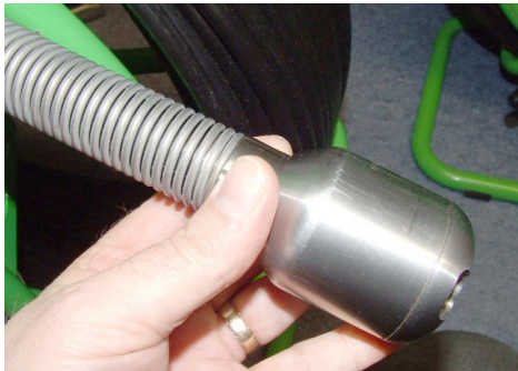
Fit camera to Rod Termination
