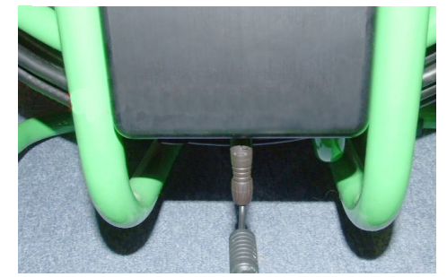
The Power Cell can be charged whilst fitted to the frame if preferred DO NOT OPERATE DURING CHARGE
