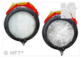
The two pipe freezing options eliminate the need to hot tap a pressurised line and reduce the cost and inconvenience of draining a pipe line
