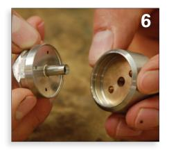
With the retaining ring removed the inlet nut will slide freely out of the body. Set the inlet nut aside. Next we will separate the head from the brass shaft. It's handy to use a vice for this next step.
