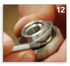
The last two steps are to re-mount the retaining ring and finally, slide the o-ring on to the inlet nut. Your **WV-P4**<sup>™</sup> disassembly and cleaning procedure is now complete. The process can be handled easily in the field or the shop. Total time to complete the cleaning is approximately 15-20 minutes.
