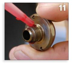
Re-assemble the *Warthog*\* following steps 2-10 **in reverse order**. Be sure to apply red 'loc-tite' to the head, (2 drops 180° apart, as shown above). When performing this step do not overtighten the head into the shaft. 100 inch-pounds of torque is sufficient.
