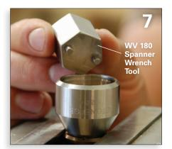
Place the body into a vice with the head down. There are two wrench flats on either side of the head. Make certain the flats are positioned properly in the vice. Next, take the WV 180 ( spanner wrench tool shown above) and set it into the two holes in the brass shaft.
