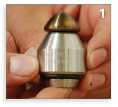
The **Warthog**<sup>®</sup> **WV-P4**<sup>™</sup> is a low maintenance tool. There are no bearings, seals or viscous fluid to replace. There are however, times when you'll want to disassemble the tool and clean it. This sheet details how to perform this operation. A flat-head screwdriver and a vice are the only tools necessary to complete the task.
