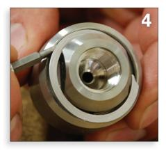
Once that is accomplished, gently rotate the tool while continuing to slide the screwdriver along, lifting the retaining ring out of the groove until it pops out completely. The ring comes off similar to a key sliding off a set of car keys.
