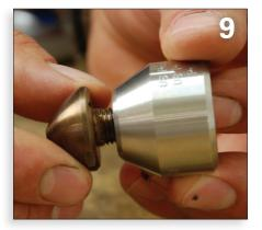
Finish unscrewing the head by hand. Remove the head and set aside. Make certain the head is clean and the drilled nozzles are free of debris. If necessary use a straight pin to clean out the drilled orifices.
