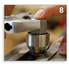
With your index finger applying downward pressure on the WV 180 spanner wrench, use a crescent wrench to loosen the shaft from the head in the vice. When reversing this step in re-assembly, do not overtighten the head into the shaft. 100 inch-pounds of torque is sufficient.
