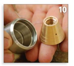
With the head unscrewed the brass shaft will drop out of the body and the disassembly process is complete. Clean all the parts. Use solvent, compressed air and a pin if necessary.
