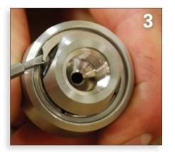
The retaining ring sits in a groove on the inside of the body. To remove the retaining ring locate the end of the ring and, with a flat-head screwdriver, separate the retaining ring by lifting the end out of the groove as shown above.
